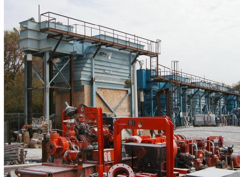
Clarifier (and filter press, if needed) for total suspended solids removal
