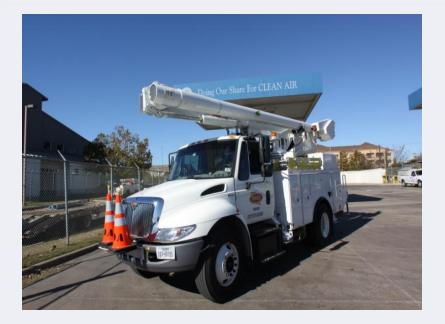
Hydraulics are battery operated
