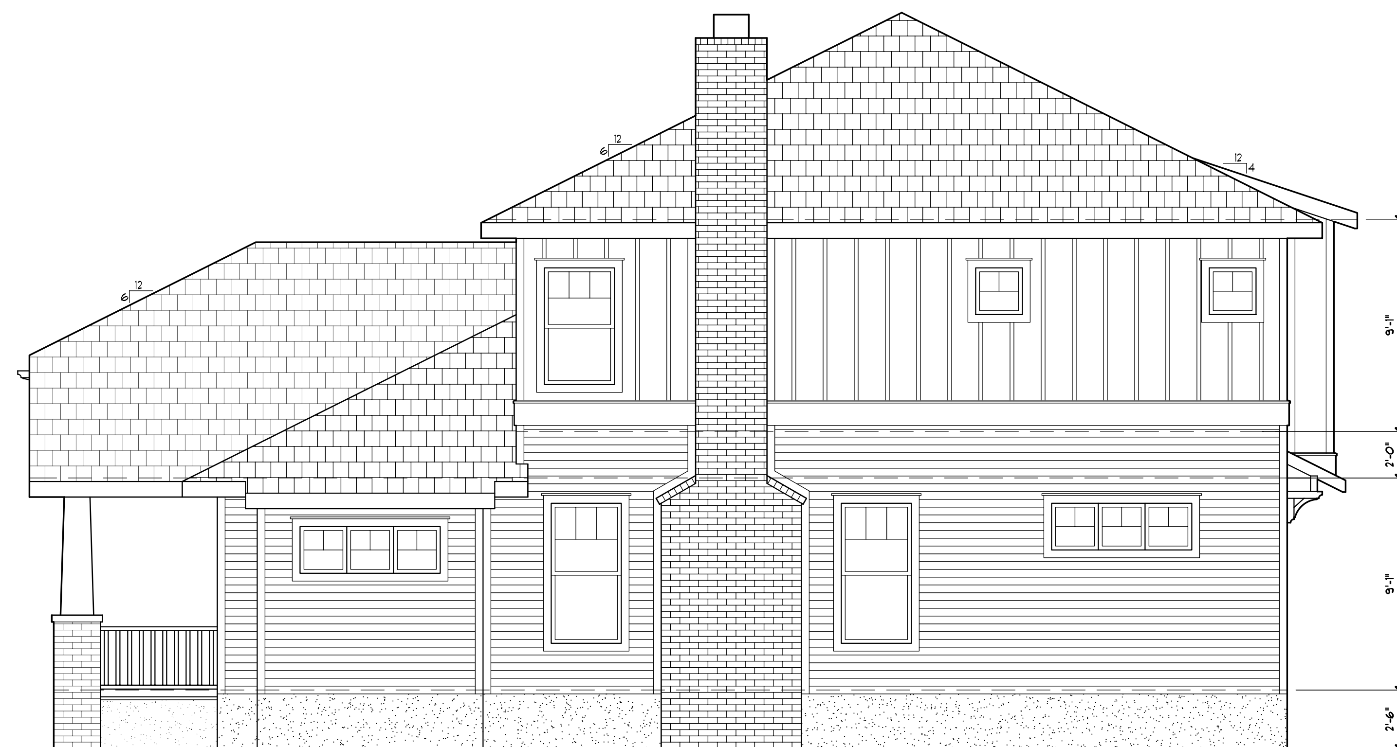
RIGHT SIDE ELEVATION SCALE: 1/4" = 1'-0"
