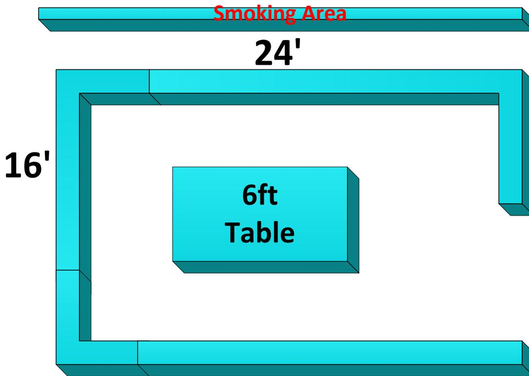
The Smoking area is constructed from 8'w x 4'h metal bicycle racks. Inside the area will be one 6' table with a total of ten urns used to both put out and dispose of cigarette butts. On the exterior Southern area of the bicycle rack a banner will be placed that reads "SMOKE HERE ONLY". An attendant will be assigned to maintain the area.
