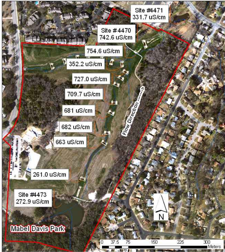
Figure 1 The Specific Conductivity increases with downstream flow until below the pathway at site 4470.
