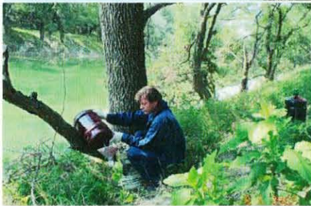
Figure 3: Vortex formed above Cripple Crawfish Cave (top). Nico Hauwert pouring eosine into a pipe inserted into Cripple Crawfish Cave on Onion Creek.
