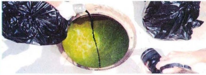
Figure 2: (left) Concrete vault and valve system above Antioch Cave within Onion Creek. (above) Sodium fluorescein dye being poured into the top of the vault.
