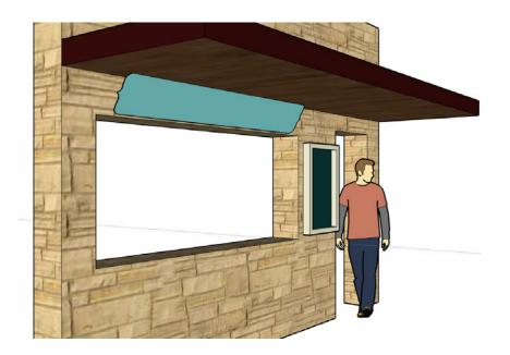
This sign will be installed above the cashier's window at the main entrance to the pool. It will be secured at and angle so that it is easy to read standing at the window. It will be secured with angled brackets.
