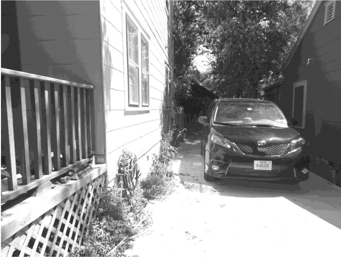
B. The space between the driveway and the ramp that leads from the existing one-car carport at the rear of the house is insufficient for the ramp to open and a wheelchair user to exit. The distance between the side of the van and the existing wheelchair ramp is about 6-1/2 feet. In addition, a large mature pecan tree at the rear corner of the house blocks a portion of the space next to the driveway.
