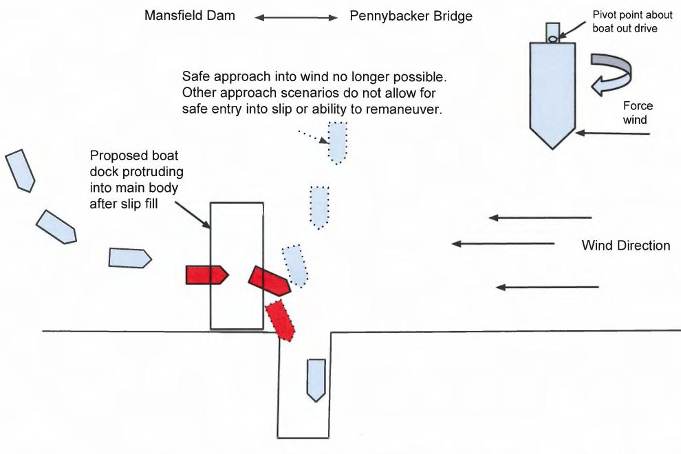
Proposed Arrangement, Entering Slip with safe and controlled entry Into Wind Not Possible Direction From Up Lake
