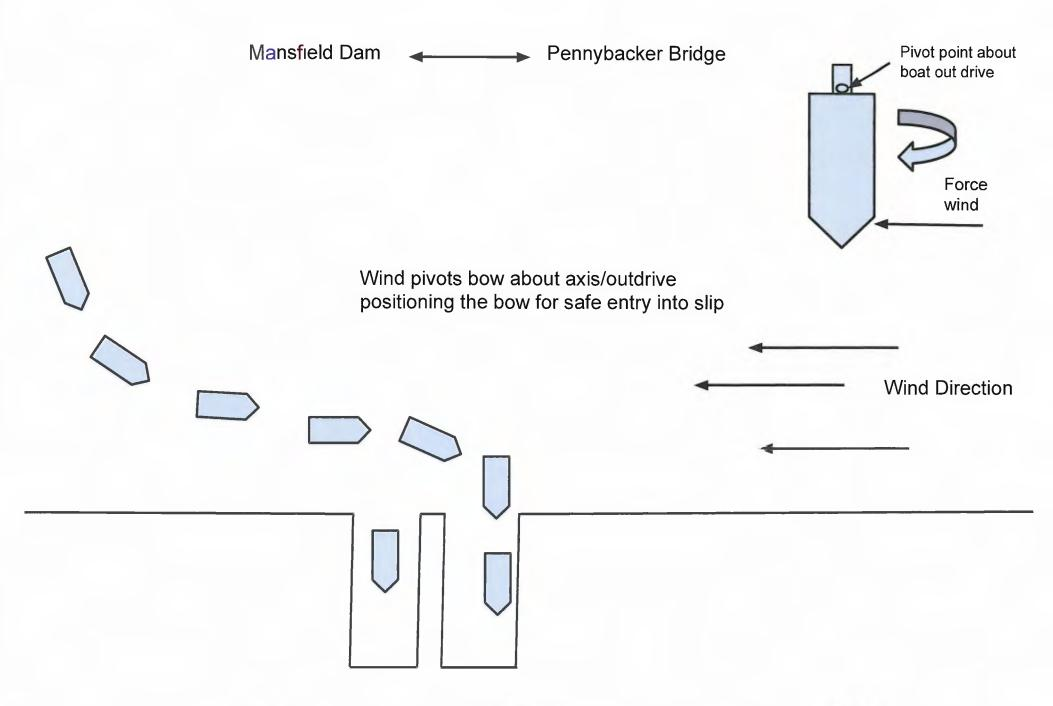
Boat Slips Today, Entering Slip Safe and controlled entry Into Wind Direction From Up Lake
