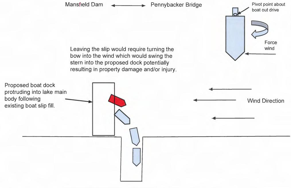
Proposed Arrangement, Existing slip filled and proposed boat dock protruding into main body. Leaving slip requires unsafe maneuver turning the bow into the wind.
