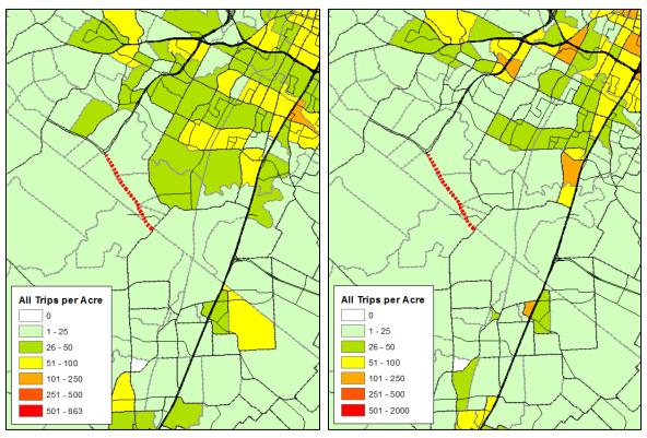
Figure 8 - All Person and Vehicle Trip Origins and Destinations by Traffic Analysis Zone (Origins, left and Destinations, right)
