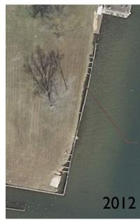
Shoreline has eroded behind existing bulkhead in 2012.
