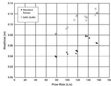
Figure 1: Head loss vs flow rate in a 4 x 4 ft sump with and without the SAFL Baffle (from Howard et al. 2011).
