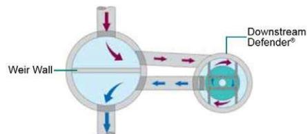
Figure 2: Downstream Defender alternate configuration (from O&M Manual linked above)
