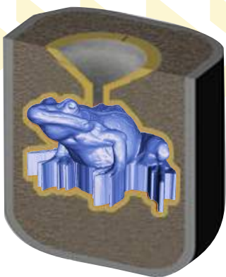
traditional fireproof mold made from cast wax model using lost wax method
