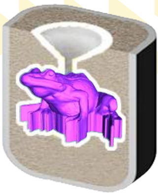
traditional rubber mold made from 3D-printed high resolution acrylate or plastic print
