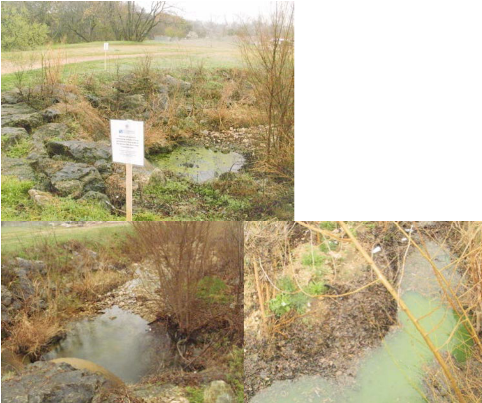
Figure 4. Photos taken of the Little Zilker Creek swallet and channel downstream near Old Mill Springs on February 26, 2014. Note the green tint of pyranine dye that was washed downstream by floodwaters in the evening of Tuesday February 25 and morning of February 26, 2014. The stormwaters likely washed a large portion of the injected dye downstream to the Colorado River before it could infiltrate into the Little Zilker Creek swallet as planned. The 2 cm (0.8 in) rain did activate springflow in the South Zilker tributary so that monitoring was initiated there February 26, 2014.
