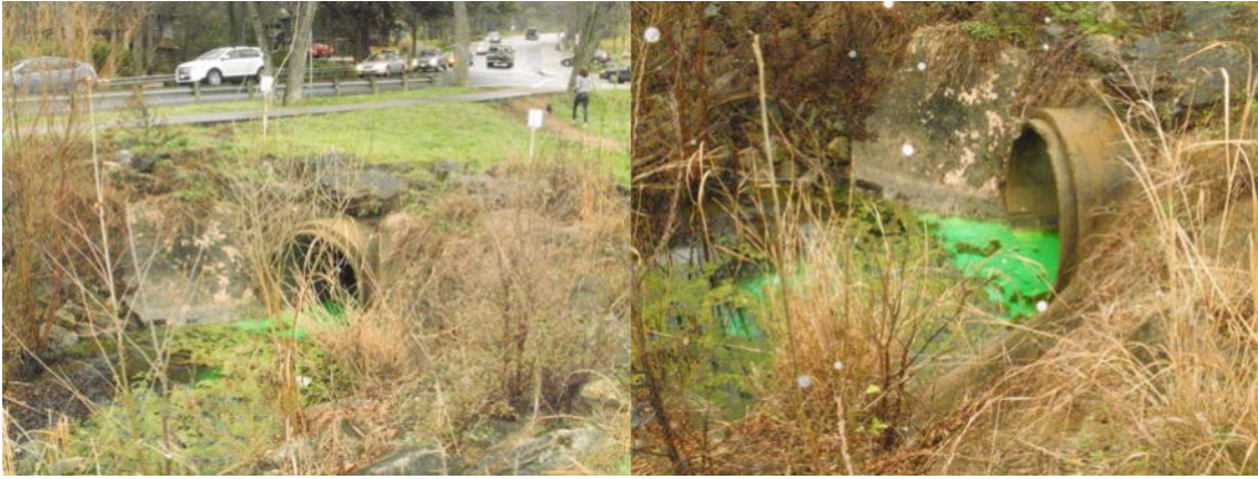
Figure 3. Pyranine was reinjected into the culvert under Robert E. Lee Road on February 25, 2014 at 8:30am. Signs were placed to alert the public for the cause of the green tracer. Flow did not extend beyond the swallet pool at the time of injection.
