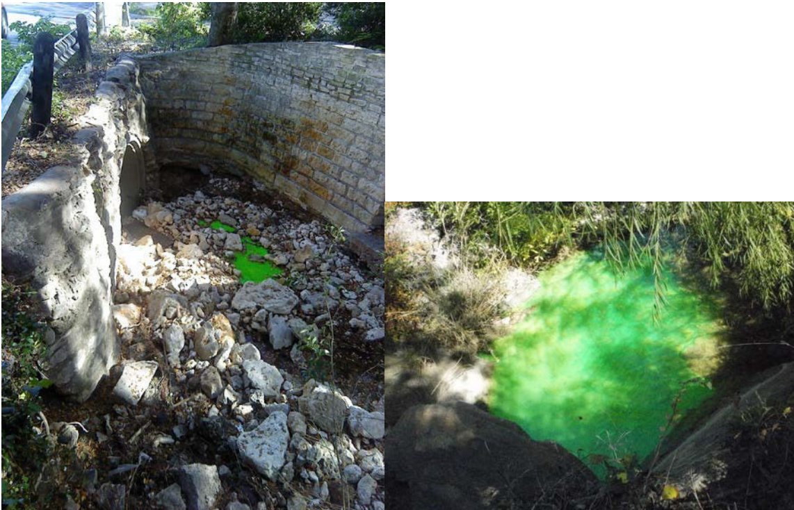
Figure 2. November 19, 2013 photos showing the tracer injection site in Little Zilker Creek upstream of Robert E. Lee Road (left photo) and the downstream swallet pool colored green with pyranine dye.
