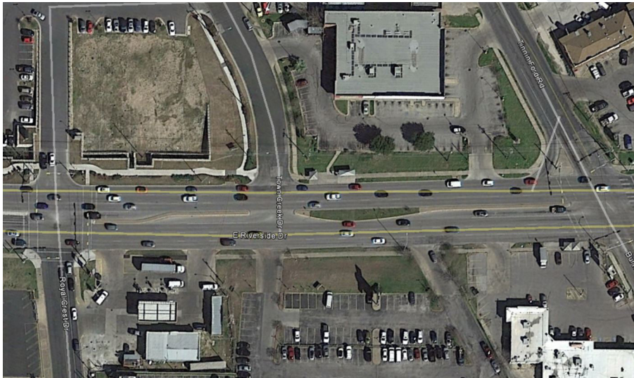
Riverside Drive T intersection with stop sign control, aligned with private drive
