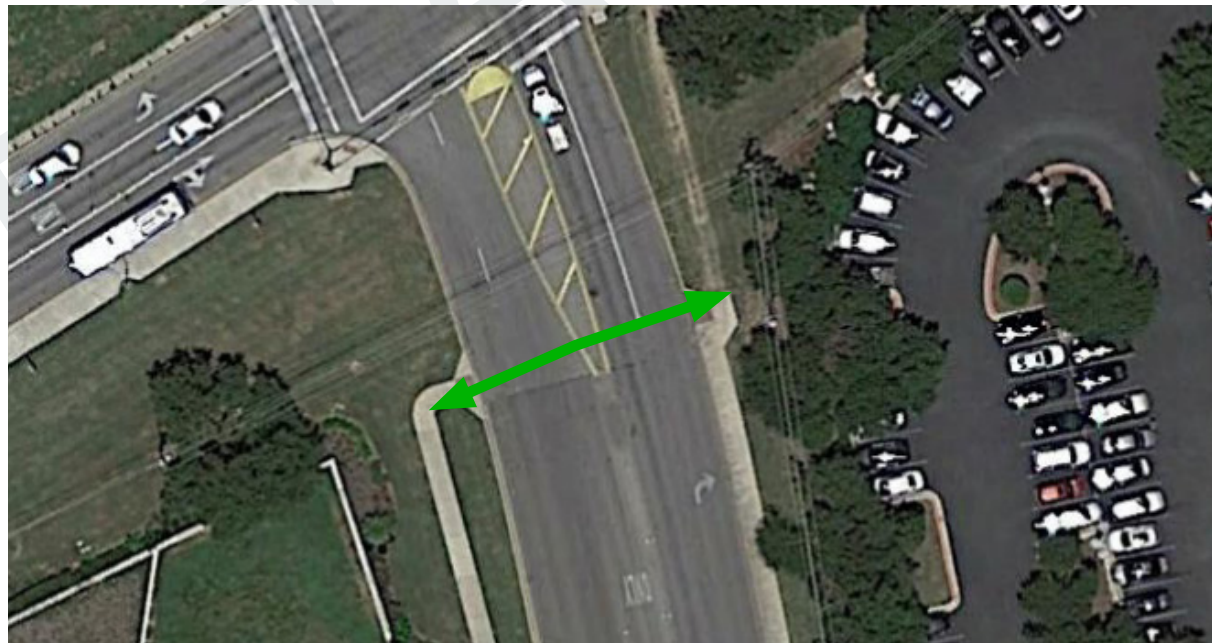
For example, this instance does not form an unmarked crosswalk (MoPac and Barton Skyway)
