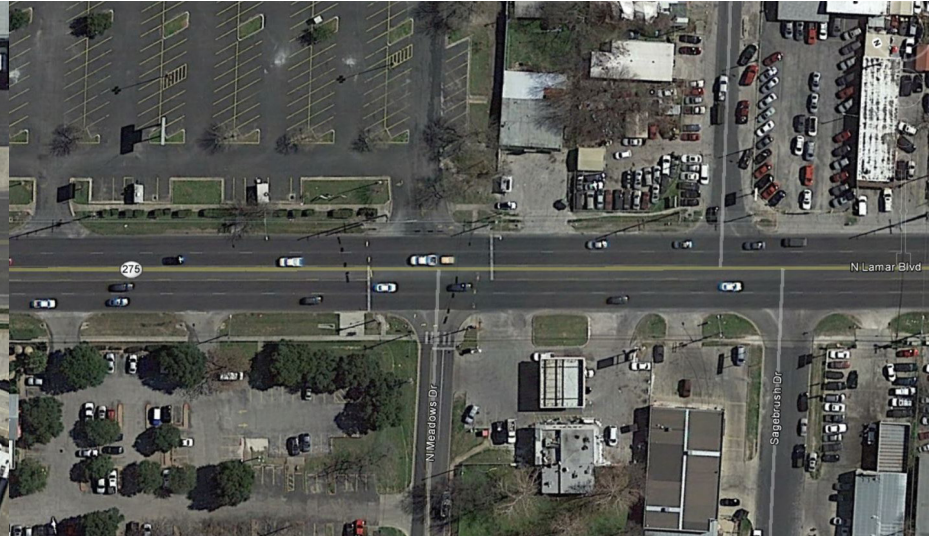
North Lamar Boulevard. Signalized T intersection with no marked crosswalk
