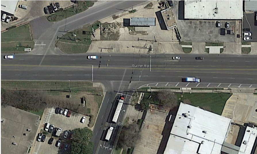
Burnet Road signalized T intersection with no marked crossing.
