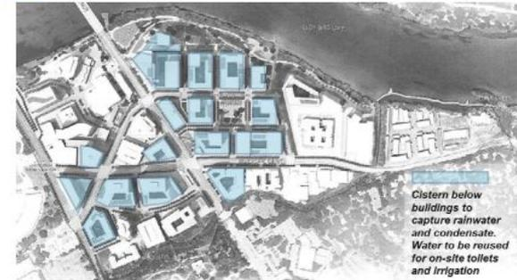
Cistern below buildings to capture rainwater and condensate. Water to be reused for on-site toilets and irrigation
