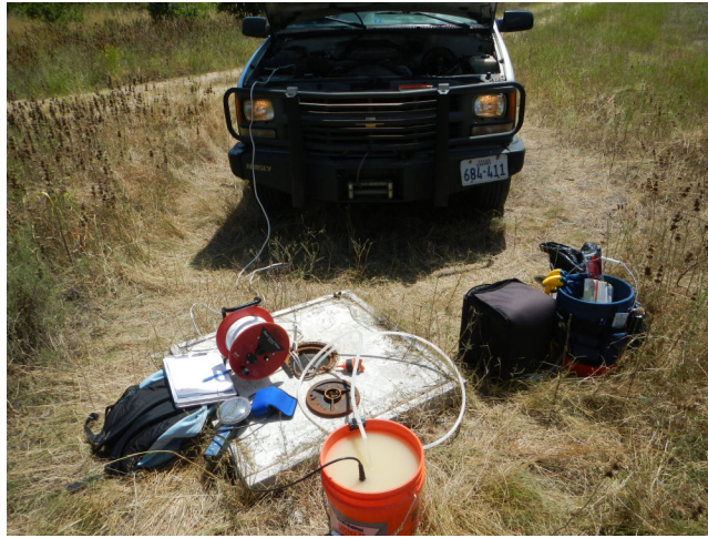
Photo 1. A typical well sampling setup (for JT108A in this case) with running vehicle supplying power to a downhole pump, an eline to monitor water levels, discharge water collecting in 5 gallon bucket to measure volume and multiprobe measuring field parameters. Car batteries were quickly drained by the pumps. Note the turbid water during the initial purging of this well.
