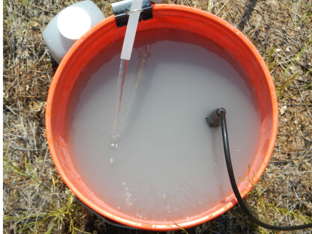
Photo 5A. Initial water pumped from JT107PZ-A shows a dull gray color indicative of the host Glen Rose limestone and marl and due to fine cuttings left over from well drilling.
