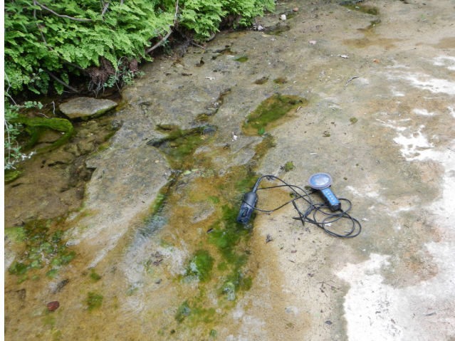
Photo 3. Groundwater from Pit Spring discharges from outlets in the alluvial bank as seen on the upper left as well as solutional openings in the channel bedrock where the multiprobe water quality sensors measure field parameters that include temperature, pH, specific conductance, dissolved oxygen, and turbidity.
