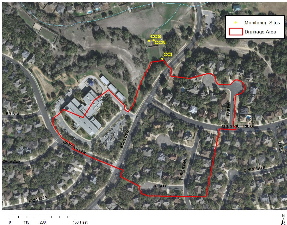
Figure 1. Canyon Creek stormwater control measure drainage area.
