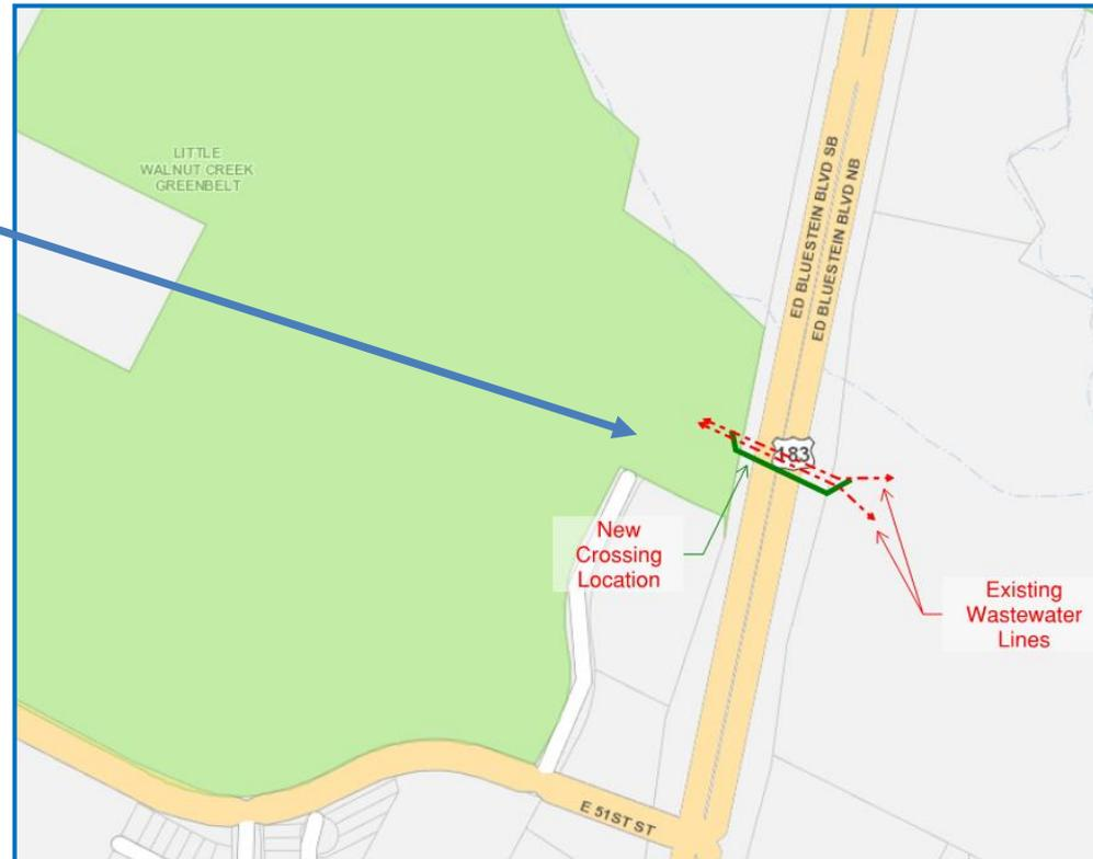
**Project Need:** This project is part of a larger utilities relocation project related to the 183 South Project in East Austin. Part of the relocations includes installing a new 72” wastewater line to replace two existing wastewater lines crossing under US 183 south of Little Walnut Creek. The majority of the work will be completed within State Right-of-Way, however additional easement is needed to tie the new 72” line into the existing wastewater lines.
