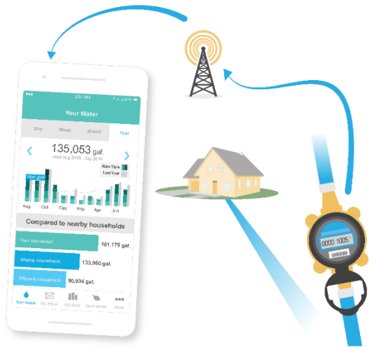
Advanced Metering Infrastructure
