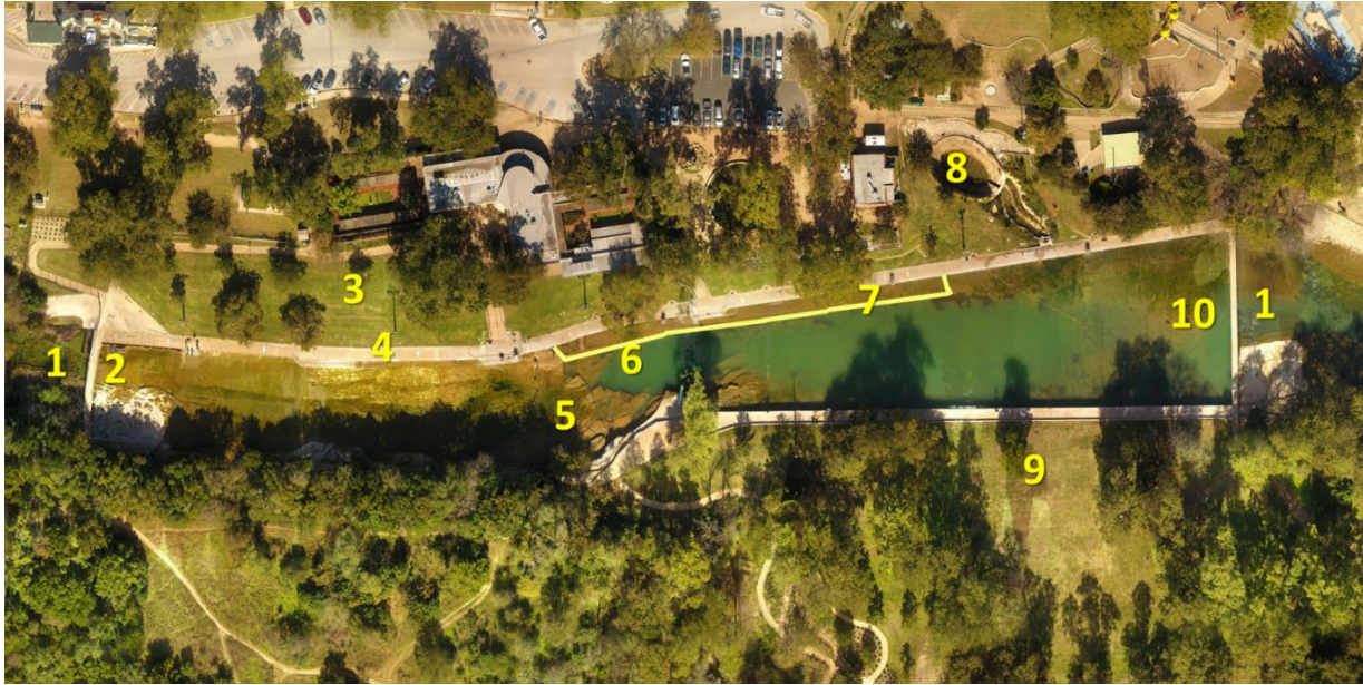
Figure 1. Aerial view of Barton Springs Pool during a full drawdown. Labels indicate: 1 Barton Creek, 2 upstream dam, 3 north lawn, 4 sidewalk with bypass tunnel underneath, 5 fissures, 6 Parthenia spring, 7 beach habitat (outlined), 8 Eliza spring, 9 south lawn, 10 downstream dam.
