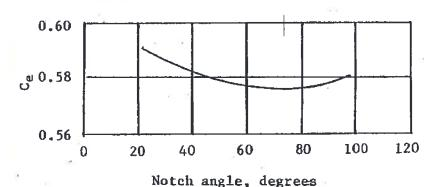
Weir Coefficient for V-notch weir Equation 8-2
