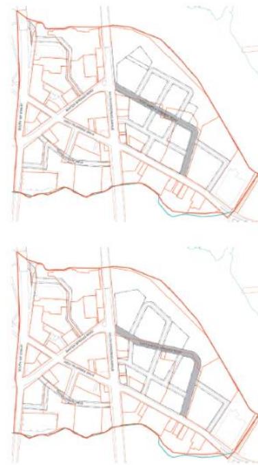
Figure 3: Possible Alignments of Barton Springs Road Extension
