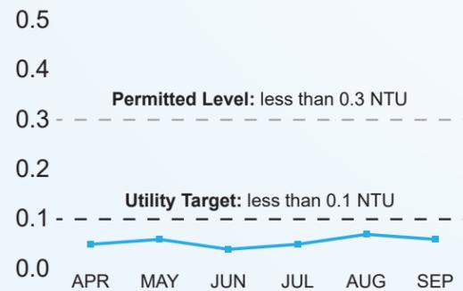
Measured turbidity "cloudiness of water" is the indicator of the effectiveness of our filtration systems. Our target is to keep treated drinking water turbidity level at 0.10 Nephelometric Turbidity Unit (NTU) or less.
