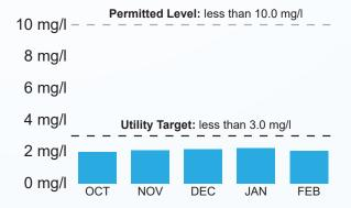
Keeps the Carbonaceous Biological Oxygen Demand (CBOD) concentration from our wastewater treatment plants discharging at 3.0 mg/L or less.
