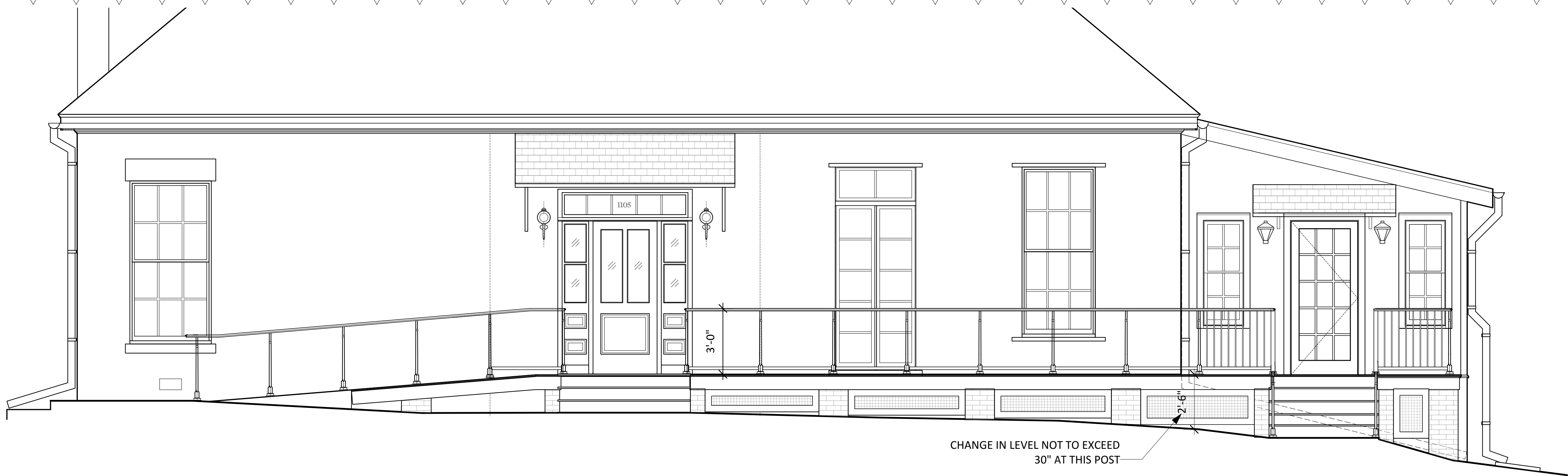
SOUTH RAMP AND ENTRY DETAIL Scale: 3/8" = 1'-0" 2
