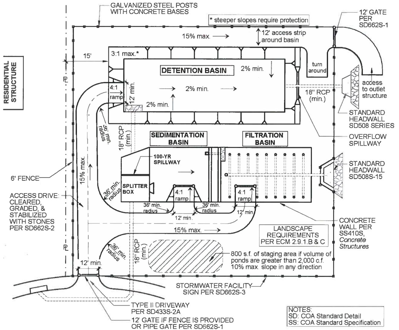
1. **Access** - This section provides the minimum requirements for reasonable access into SCMs for maintenance and inspection activities for both residential and commercial developments.
