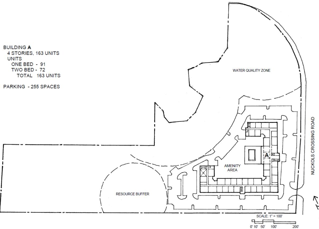
\* Access location approved by ATD after survey, sight line, and speed analyses for ATD. Location will likely require associated safety improvements (right-turn bay, left-turn lane, etc.) for site plan approval.
