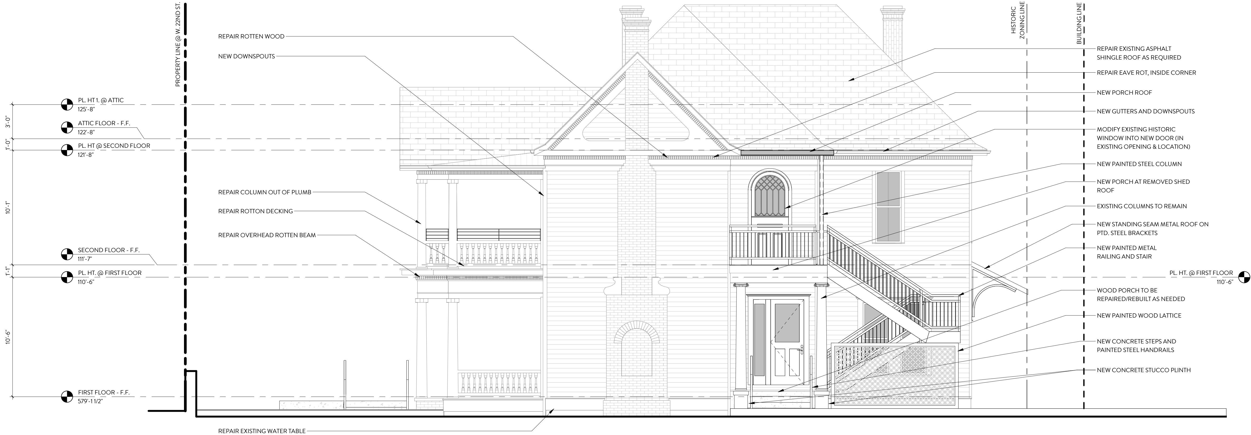
2 WEST ELEVATION - RIO GRANDE STREET ENTRY - PROPOSED 1/4" = 1'-0"
