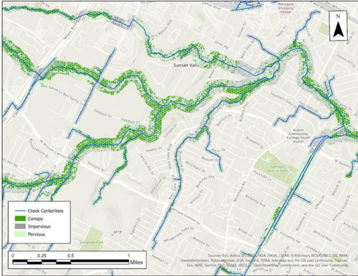
Figure 4. Example map showing the individual categories of canopy (dark green), impervious cover (grey), and pervious cover (light green) distributed throughout the entire buffer/hexagon network.
