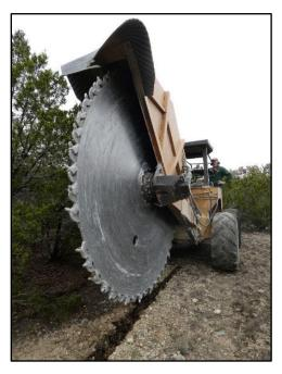
A giant rock saw was used to trench around an oak wilt center found on the Steiner Ranch conservation easement, as well as the City of Austin's Cortaña tract and the Steiner Ranch Homeowner Association's greenbelt. Trenching cuts off root contact between infected and uninfected trees to prevent further spread of the disease.
