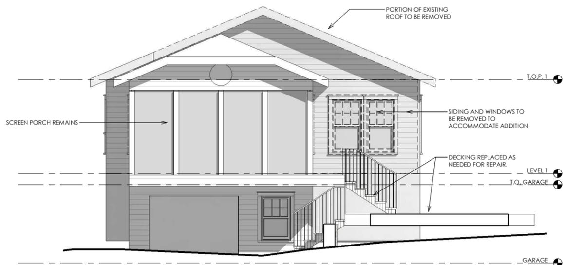
**3 DEMOLITION - WEST ELEVATION (REAR)**
