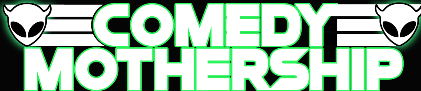
Opt 3- Aluminum painted sign can with double stroke neon to match existing- flat cut aliens with Neon All options will be attached to allow removal without compromising the historic fabric
