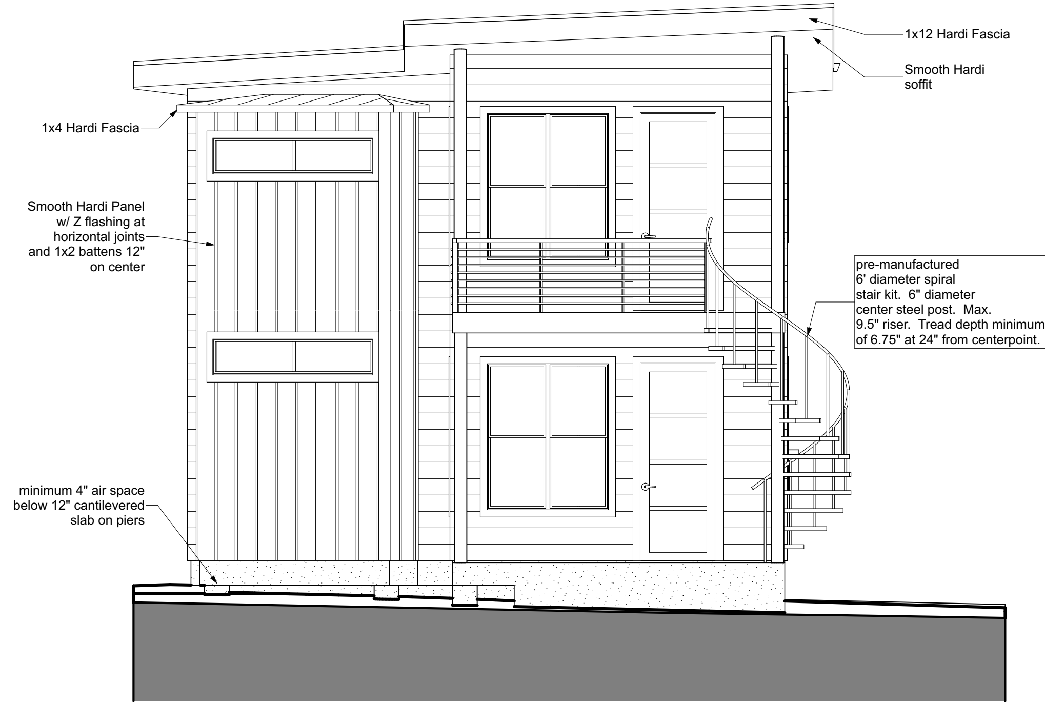
5 Front and Stair Elevation 1/4" = 1'-0"
