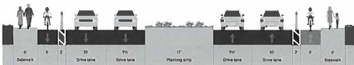
Figure 2: Existing Cross Section of Loyola Lane
