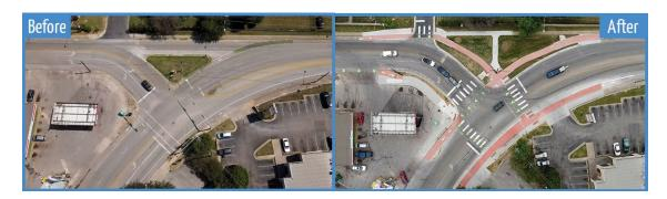
A new protected intersection is now complete at Payton Gin and Ohlen roads to provide safer connectivity for people walking, biking, and driving. The work included replacing a slip lane with a rain garden and connected sidewalk, protected bike lanes and shorter, accessible and more visible pedestrian crossings at all legs of the intersection.
