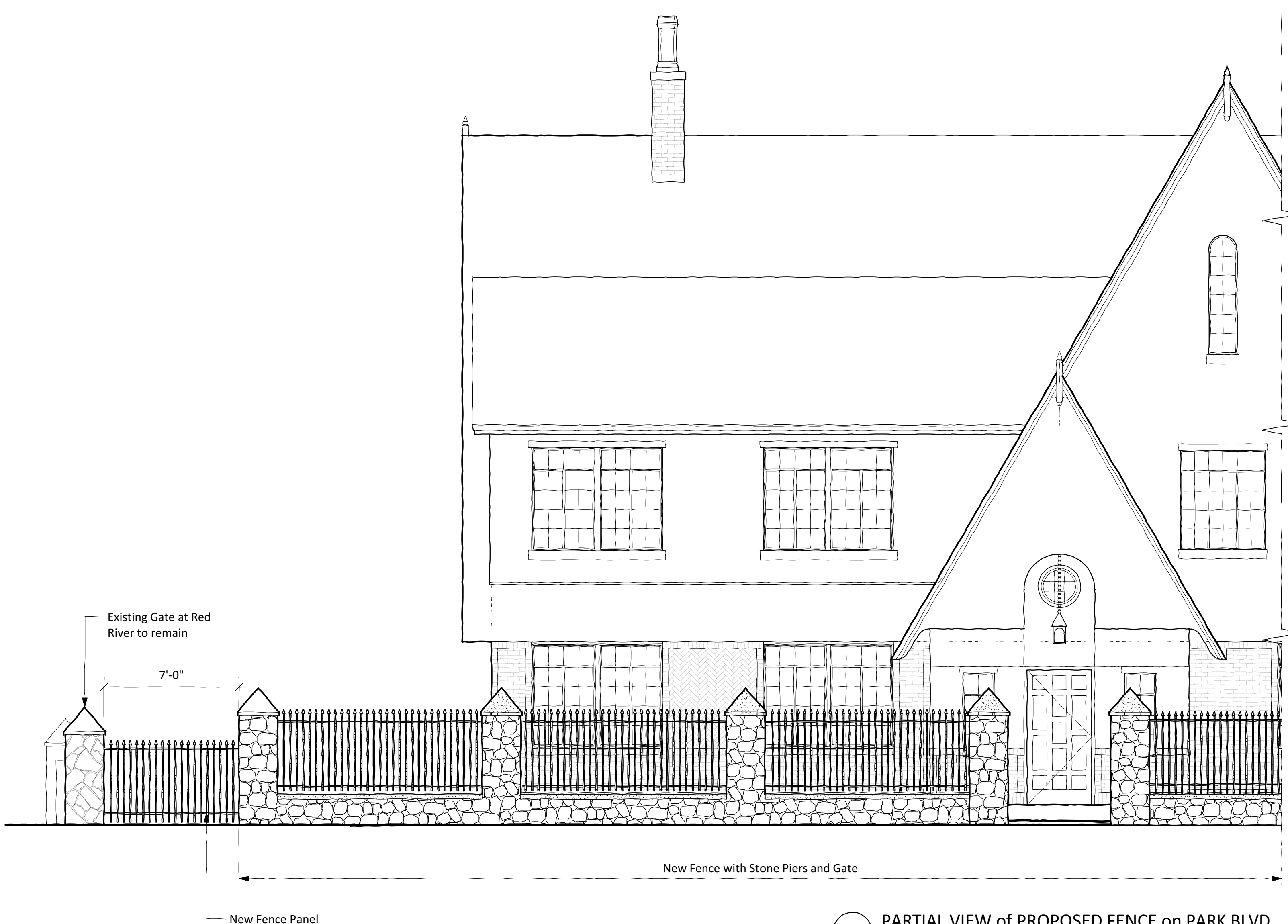
1 PARTIAL VIEW of PROPOSED FENCE on PARK BLVD. Scale: 1/4" = 1'-0"
