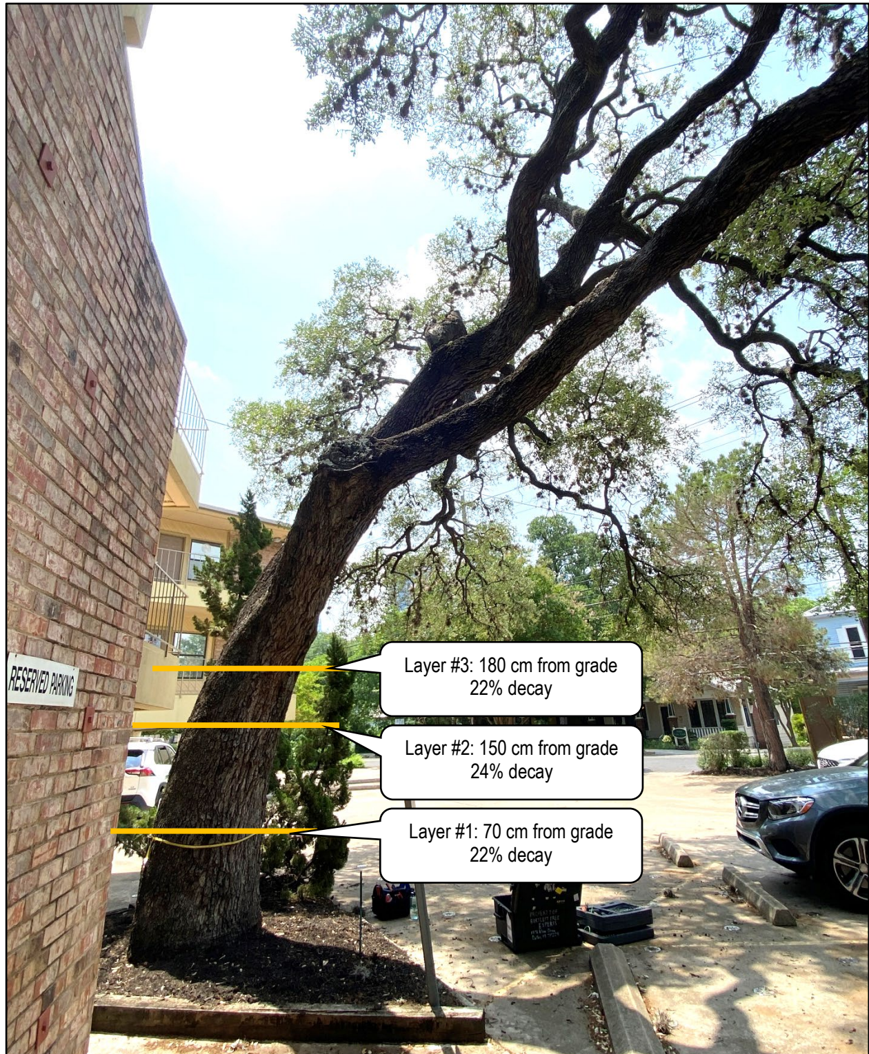
Image 5: Tree leans southwest over the parking area. Tree canopy is asymmetrical. Sonic tomography locations indicated by the yellow lines. A column of decay was located in the center of the stem. Pruning wound with decay on west stem is visible.
