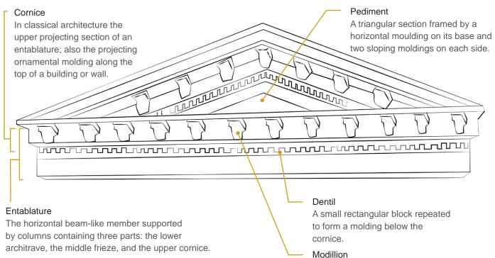
A small rectangular block repeated to form a molding below the cornice; larger than a dentil.
