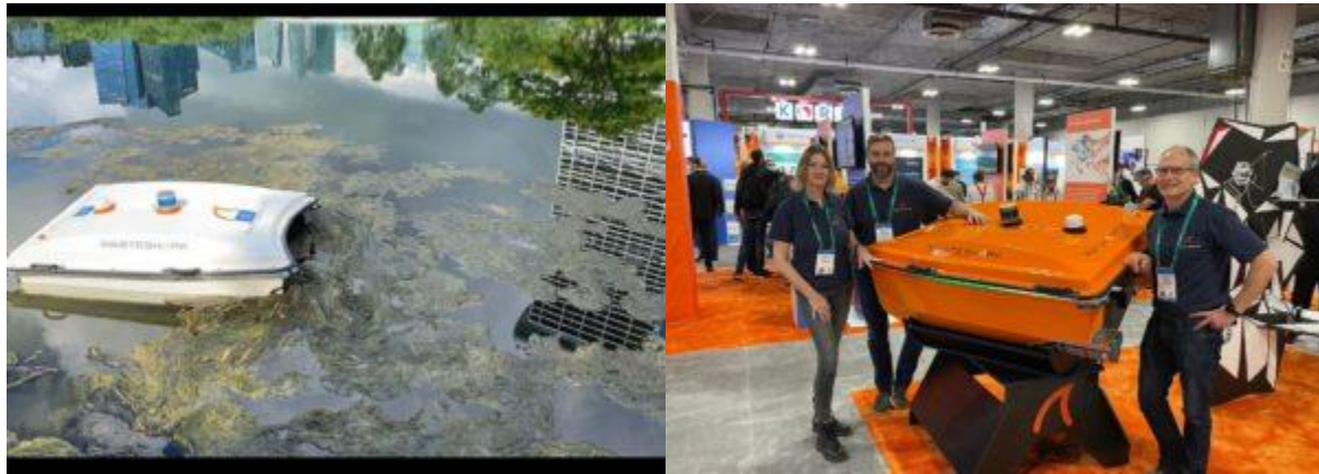
Figure 6. Waste Shark Aquatic Litter Robot and photo to show scale (Photos courtesy of RanMarine for Wasteshark photo and IADYS – Interactive Autonomous Dynamic Systems for Jellyfishbot photo)
