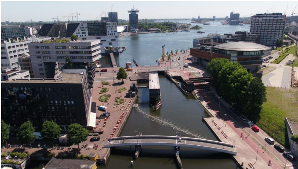
Figure 9. Bubble barrier diverting flow to Containment Trap, Netherlands ( Photo courtesy of The Great Bubble Barrier )
