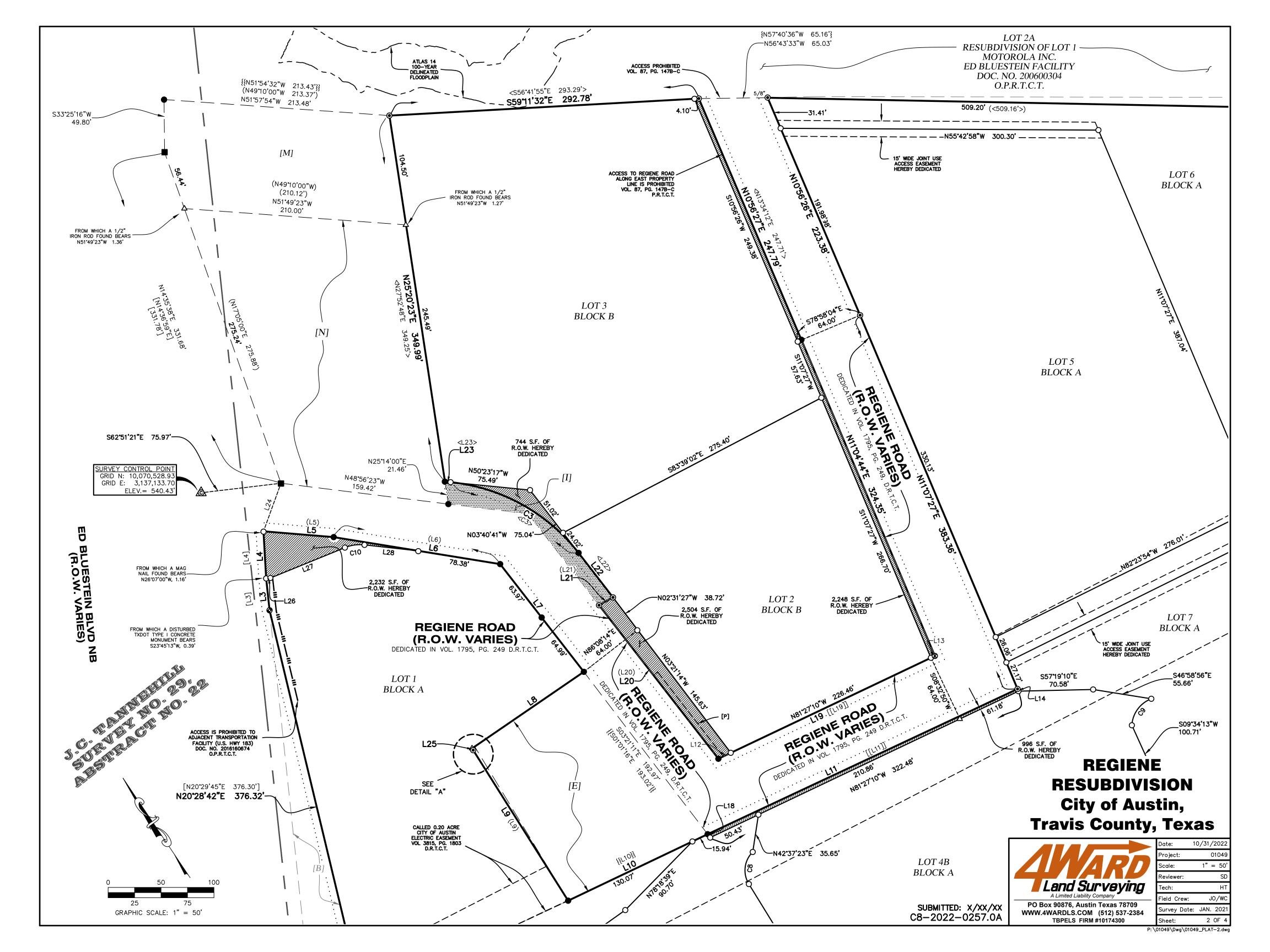
ALL BEARINGS ARE BASED ON THE TEXAS STATE PLANE COORDINATE SYSTEM, GRID NORTH, CENTRAL ZONE, (4203), NAD83, ALL DISTANCES WERE ADJUSTED TO SURFACE USING A COMBINED SCALE FACTOR OF 1.000029500981.
