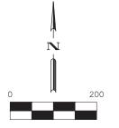
BEARING ORIENTATION IS BASED ON THE TEXAS STATE PLANE COORDINATE SYSTEM, CENTRAL ZONE 4203, NAD-83.
