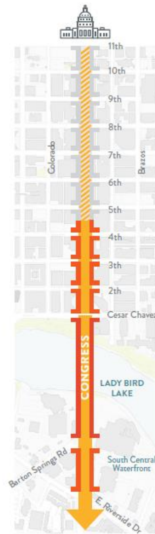
Phase 1B: Multimodal Avenue Reconstruction of intersections at Riverside Drive, Barton Springs Road, and Cesar Chavez Street. Full reconstruction of roadway from Riverside Drive to 4th Street. Maintain protected bike and scooter lane north of 4th Street.
