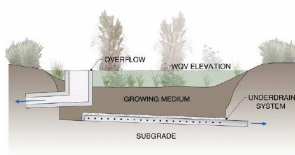
Figure 1.6.7.H-4. Full infiltration rain gardens are sized to capture and convey runoff through a biofiltration bed underlain by an underdrain system.
