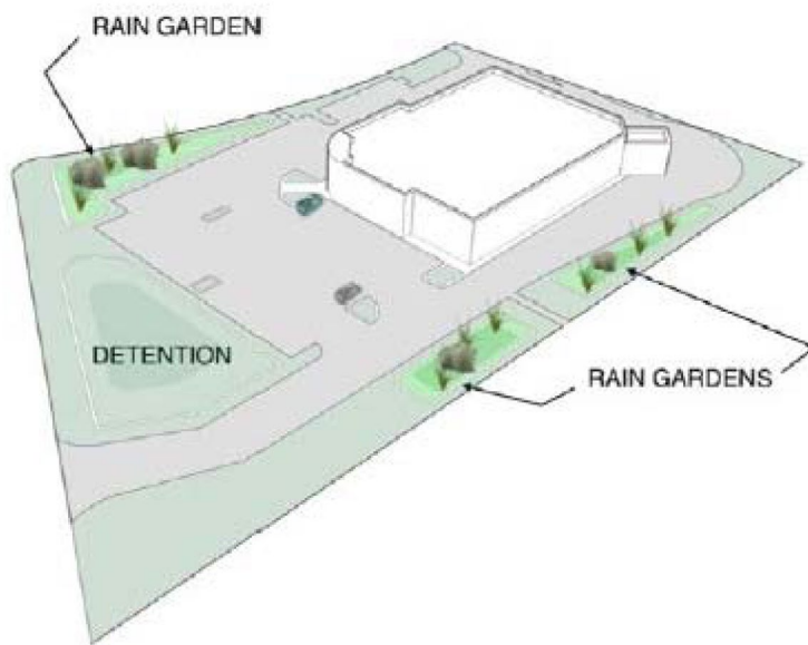
Figure 1.6.7.H-1. Multiple rain gardens may be dispersed across a development, and incorporated into the landscape, providing aesthetic as well as ecological benefits.
