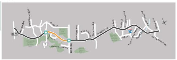
The project is sponsored by TPW and consists of improvements including the installation of one added lane in each direction (less than 18" excavation depth), traffic signal improvements at multiple locations (limited excavation), installation of shared use paths and vegetative stirps behind roadway curbs, a pedestrian hybrid beacon near Zuniga, two new water quality ponds, refurbished existing water quality
