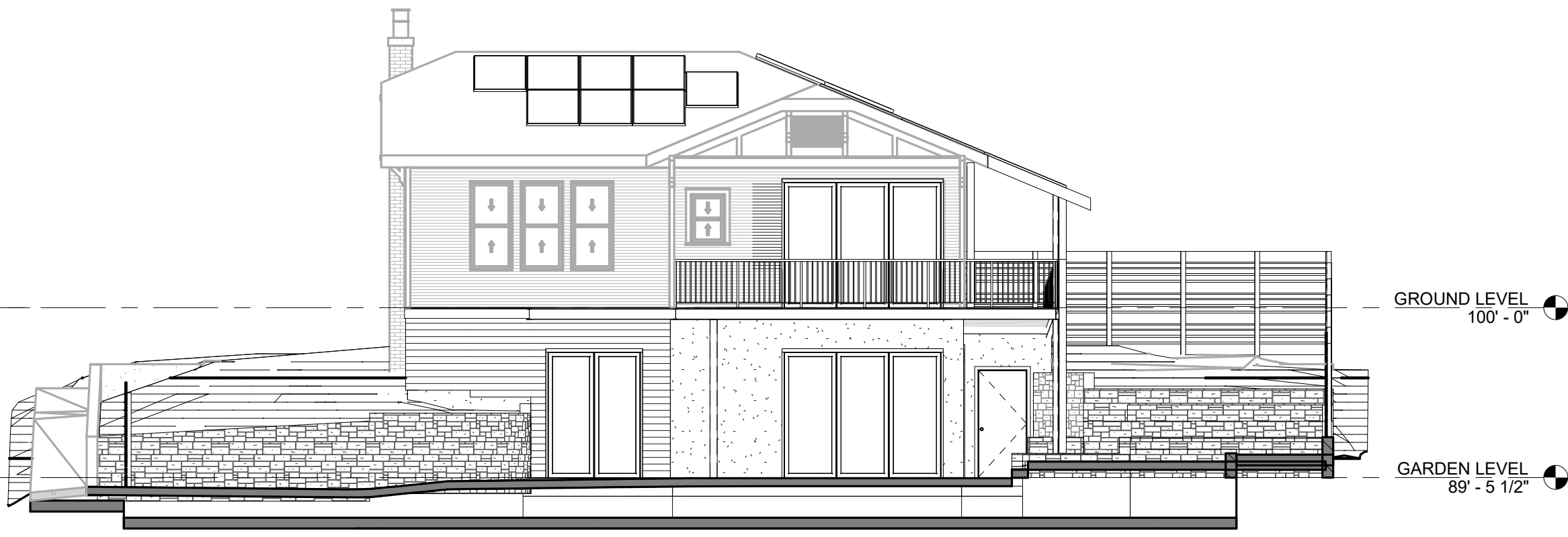
2 SUBCHAPTER F - SOUTH ELEVATION 1/8" = 1'-0"
