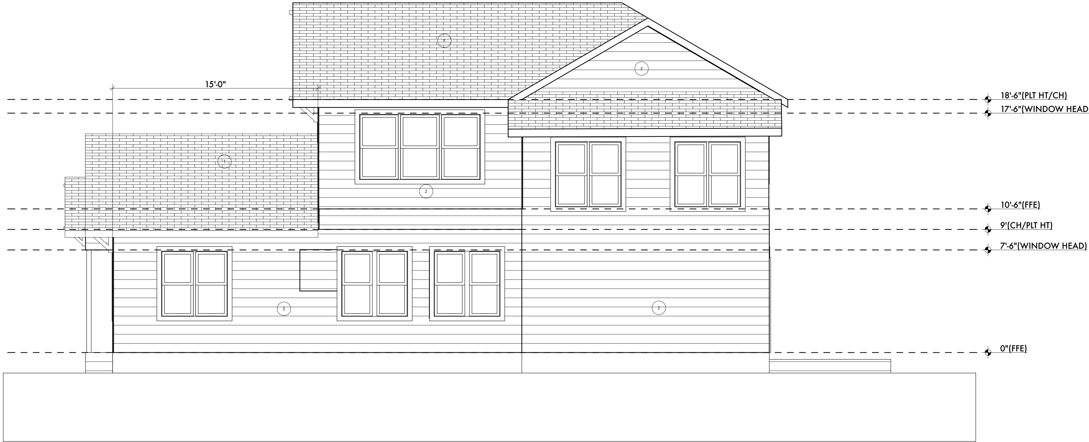
SOUTH ELEVATION SCALE: 1/4" = 1'-0"
