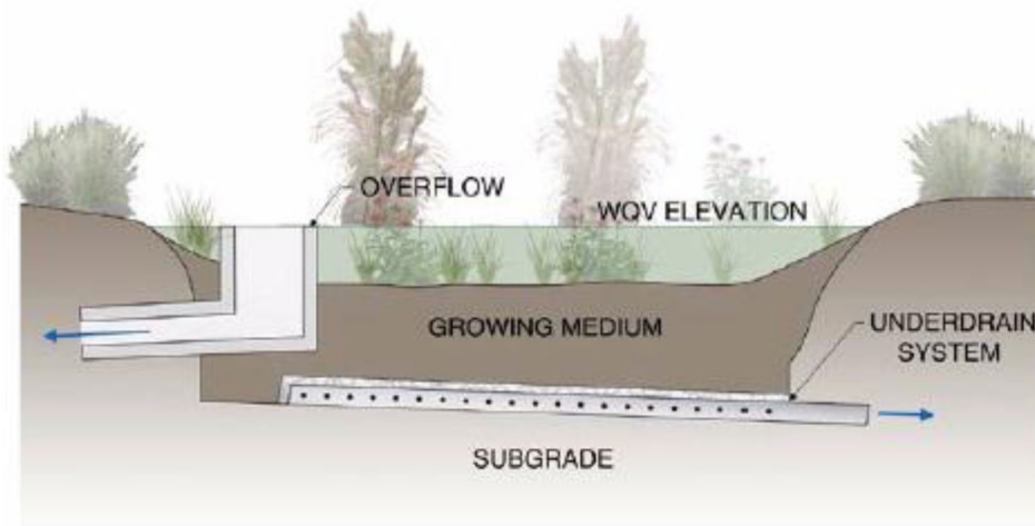
Figure 1.6.7.H-4. Full filtration rain gardens are sized to capture and convey runoff through a biofiltration bed underlain by an underdrain system.
