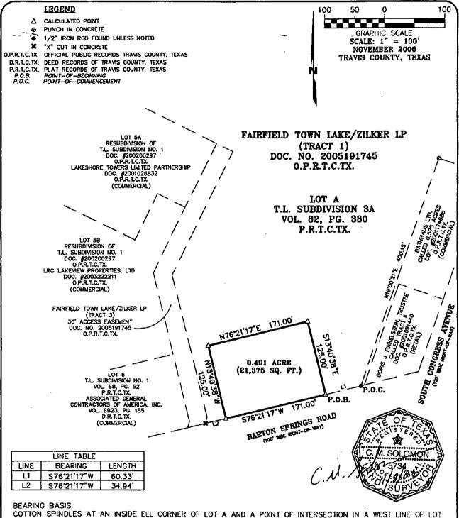
COTTON SPINDLES AT AN INSIDE ELL CORNER OF LOT A AND A POINT OF INTERSECTION IN A WEST LINE OF LOT A OF T. L. SUBDIVISION 3A, A SUBDIVISION OF RECORD IN VOLUME 82, PAGE 380 OF THE PLAT RECORDS OF TRAVIS COUNTY, TEXAS. CALLED BEARING AND DISTANCE BETWEEN THESE COTTON SPINDLES IS N26\*12'E - 228.39 FEET. HELD CALLED BEARING OF N26\*12'00"E AND FOUND ACTUAL DISTANCE TO BE 228.38 FEET.
