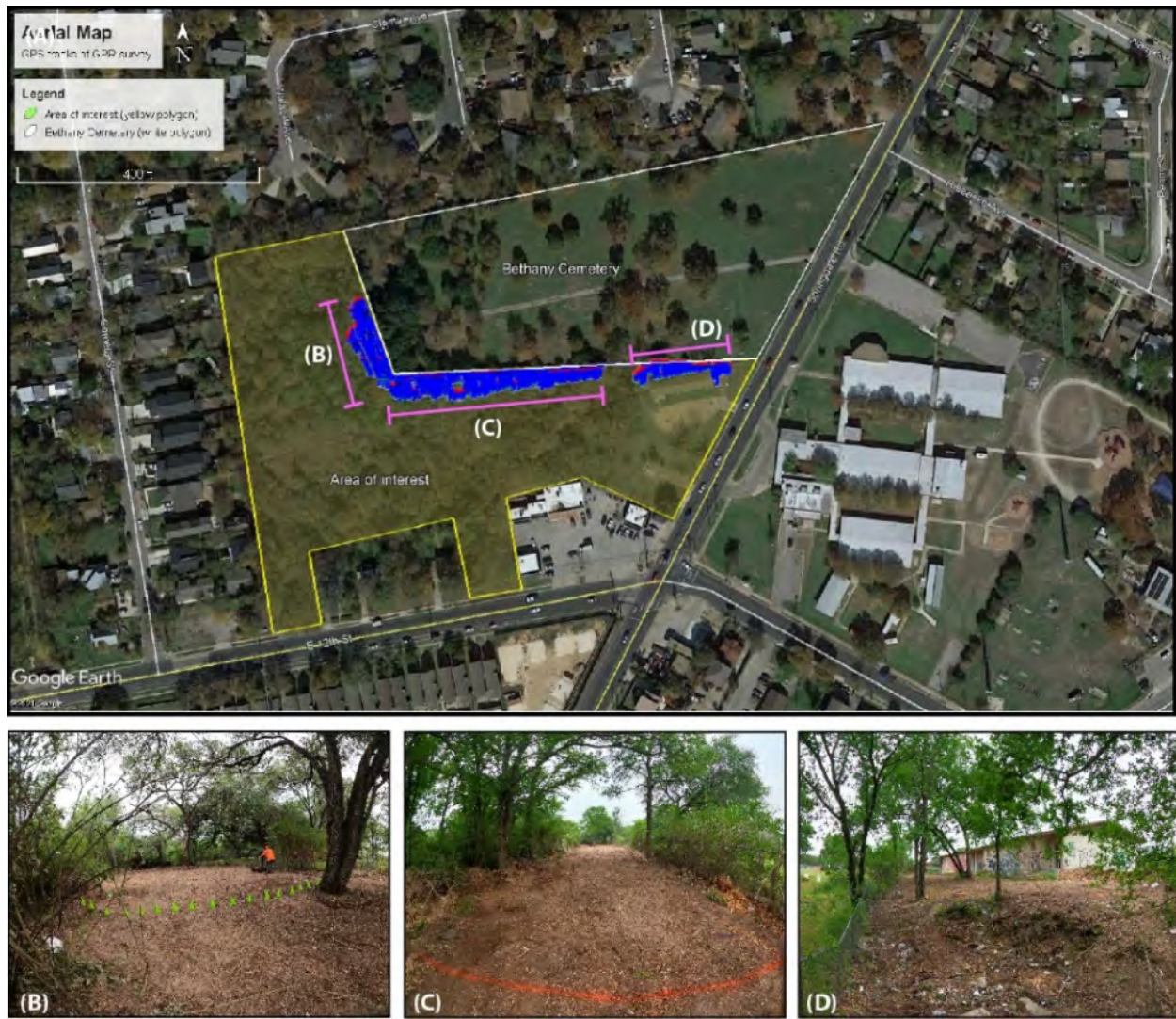
Figure 3. (A) Aerial photograph of the target area at 4120 E. 12 th Street, Austin, Texas, 78721. The GPR survey was done in an L-shaped grid approximately ~30-ft-wide by ~700-ft-long. The blue lines show the orientation of all GPR-GPS tracks during the GPR survey, which borders Bethany Cemetery's current boundary. The gap in the GPR-GPS tracks is due to the occurrence of a natural channel backed filled with trash (see Figure 3D). Field photographs are shown in (B) to (D). Photo sources: (A) from Google Earth, (B) to (D) by author.
